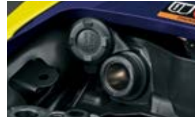
DC Socket 38800-31810-000 Gives option to customers for usage of electric devices. To be installed underneath seat.
